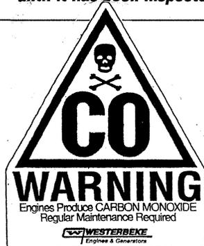
**A WARNING DECAL is provided by WESTERBEKE and should be fixed to a bulkhead near your engine or generator. WESTERBEKE also recommends installing CARBON MONOXIDE DETECTORS in the living/sleeping quarters of your vessel. They are inexpensive and easily obtainable at your local marine store.**
